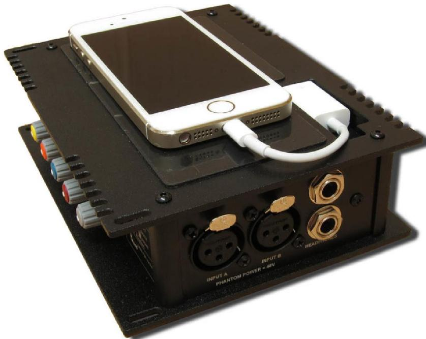
As shown in the above picture the supplied long thin converter should be used to connect to an iPhone/ iPod/ iPad with a lightning connector. The long thin converter should be inserted in the opening on the top of the CUB and it should be plugged into the USB plug located there. Please note the long thin converter has a USB socket on it and as such it can only be inserted one way up.
