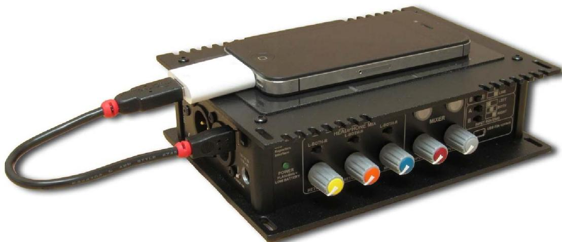
As shown in the above picture the supplied short fat converter and mini USB to USB A cable should be used to connect to an iPhone/ iPod/ iPad with a 30 pin connector.
