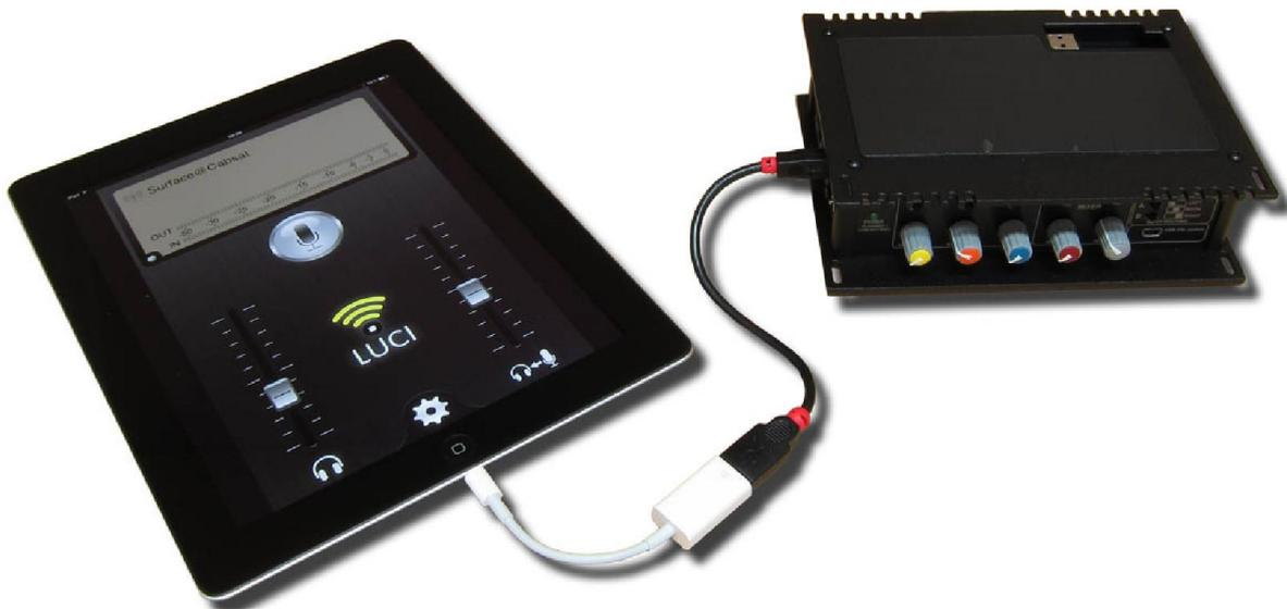
When connecting to an iPad either the short fat converter or the long thin converter will be needed. Then connect the USB A socket of the converter to the mini USB socket on the side of the CUB as per the above photo.
