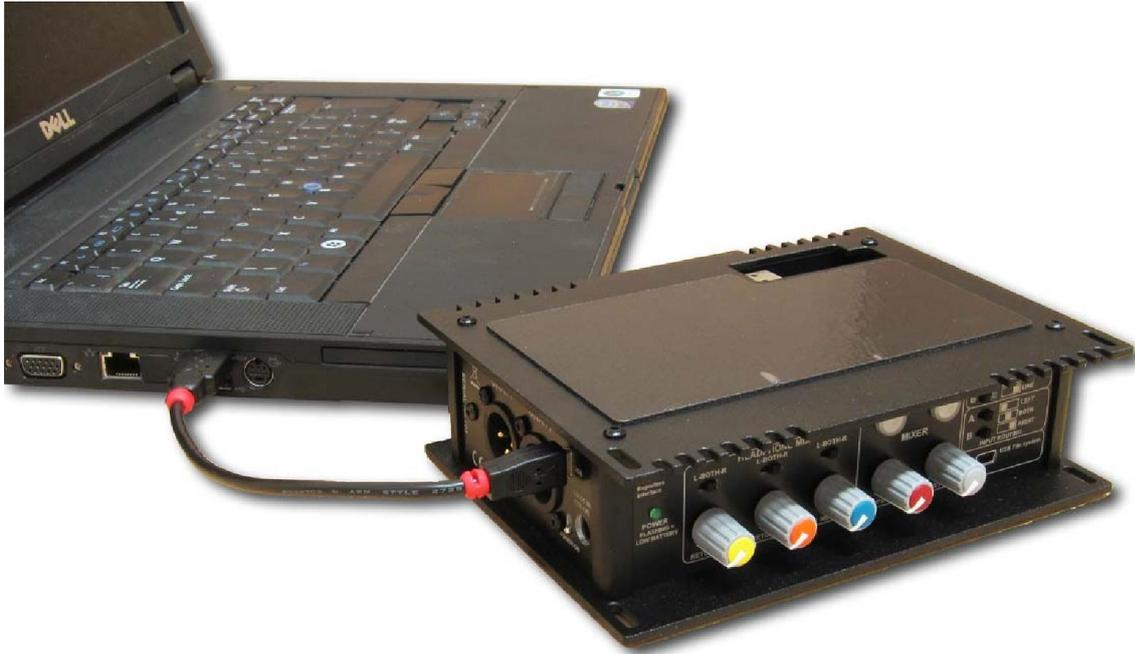
As shown in the above picture, connect the CUB to a PC using the mini USB socket on the side of the device.
