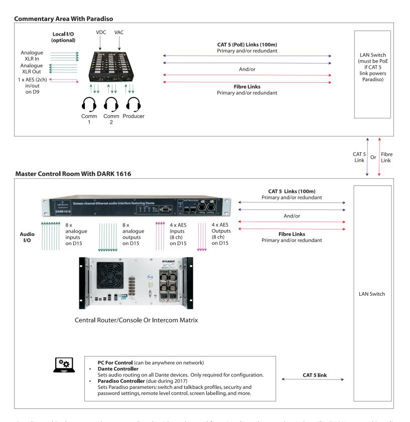
Paradiso and Dark 1616 can also connect directly without the need for going through network switches. The DARK 1616 and Paradiso can be set to operate in AES67 mode for compatibility with other AES67 units.
