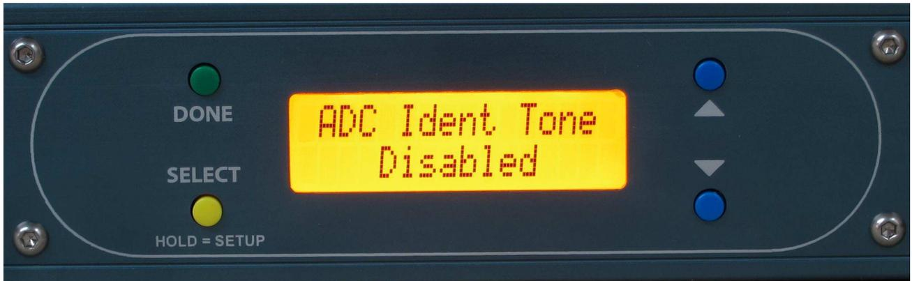
Turning on the ADC Ident tone (enabling it) adds a 1kHz tone @ 0dBu to the digital output. This can be useful for fault finding.
