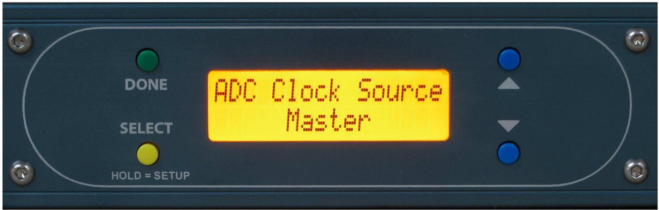
This control sets what clock source is used as a reference for the ADC. The digital output will be locked to the selected source. There are 4 options.
