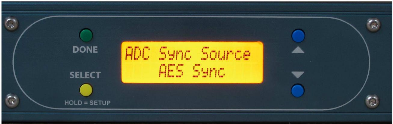
This sets which of the 3 possible external reference clock sources the device should use.
