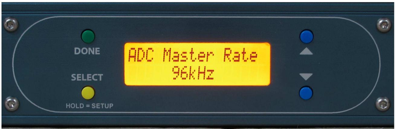
This sets the output sample frequency of the internal clock. There are 6 options:
