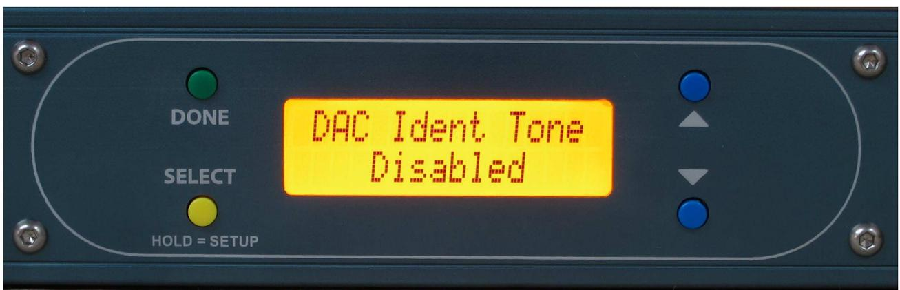
Turning on the DAC Ident tone (enabling it) adds a 1kHz tone @ 0dBu to the analogue output. This can be useful for fault finding.
