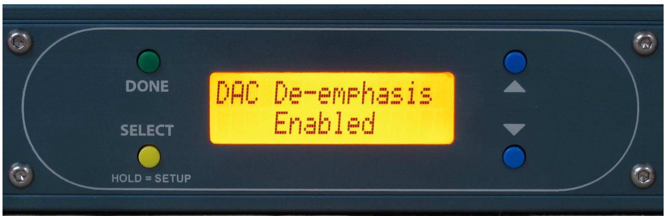
If your digital audio source was originally mastered with pre-emphasis (normally the high frequency boost) then enabling de-emphasis removes this during the D/A process.
