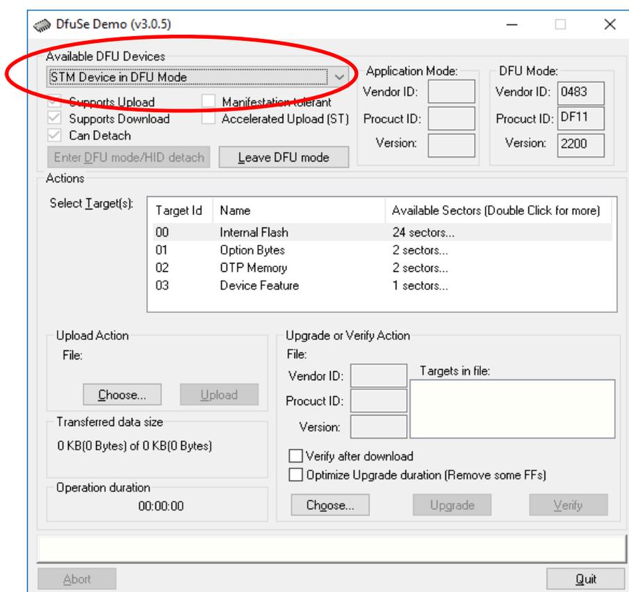
*Figure 2 Device successfully recognised*
