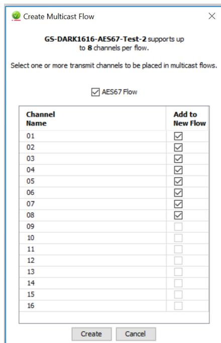
Tick the AES67 Flow check box, then select up to 4 channels to be included in the flow then click 'Create'
