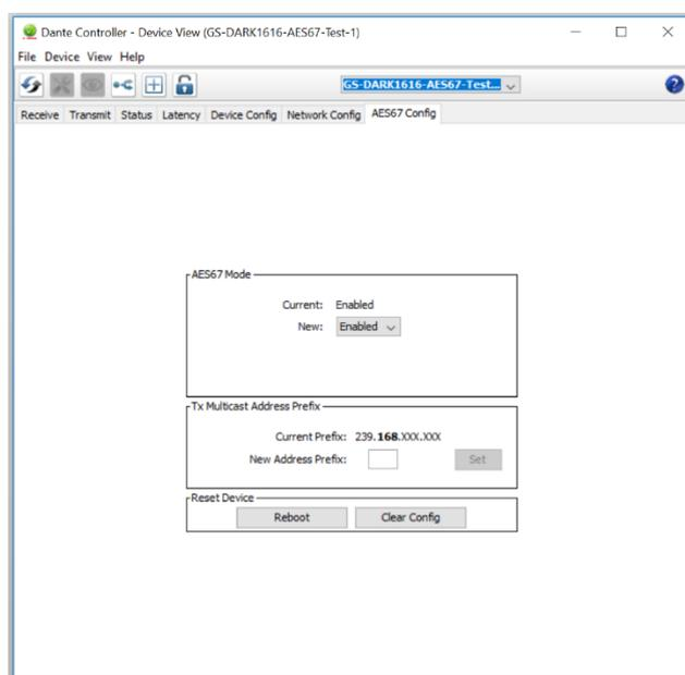
Once the AES67 drop down box has been enabled you'll have to reboot the Athens 2 for the change to take effect. After the reboot go back to the AES67 tab and set the multicast prefix address to one that is suitable for your network.
