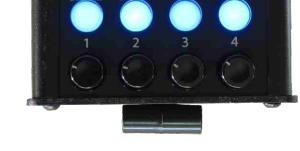
tap of any talk button will produce a 'call' signal alert that will be received by another Beatrice unit. An LED indicates an incoming call alert, which will also produce an audio indication on the headphones.
