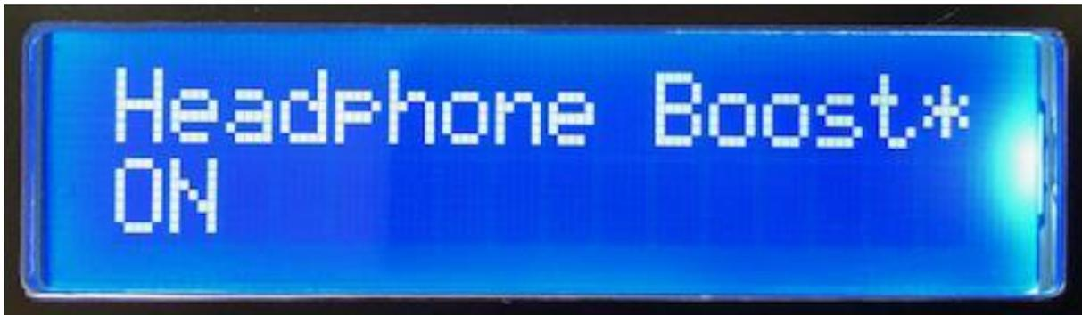
If 'ON' is not shown on the setup screen as per the above picture then headphone boost is turned off.
