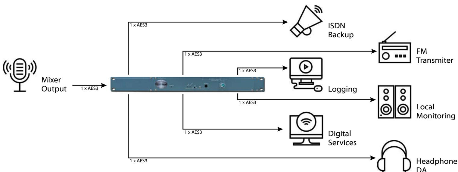
In this example, the main stereo programme feed from a radio station needs to be distributed across multiple platforms. The output from the desk or automation system no longer just heads off to the transmitter. The audio must be distributed across all of the relevant services that require a connection of the original programme audio.
