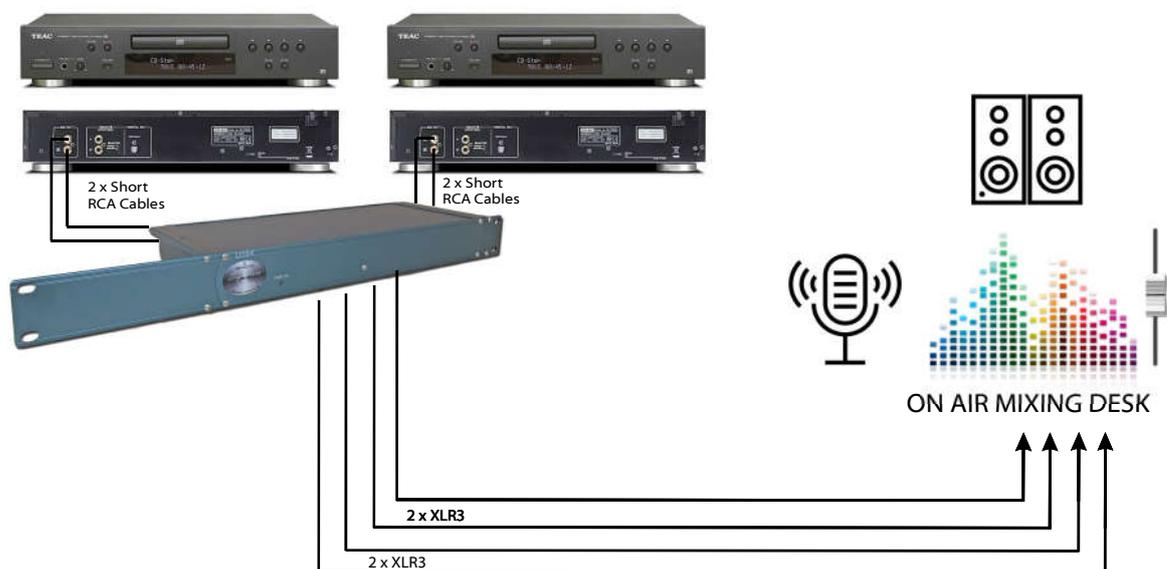
Many radio stations and studios incorporate mid level domestic audio equipment such as CD players as they provide reasonable value for money in comparison to professional versions. The output of such devices need to be correctly interfaced with a professional or broadcast audio desk. In this example the U2B4 will be located near the two CD players as it is prudent to keep the unbalanced audio cables as short as practicable.
