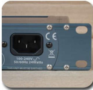
A Signature unit can be rack mounted via the front panel or if it is more convenient, via the rear panel by simply swapping the rack ears over.
