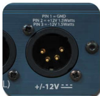
All Signature units (except PS1) have a 4 pin XLR  $\pm 12V$  DC socket for connection to the PS1 Power Station. This can act as the primary or backup power source.
