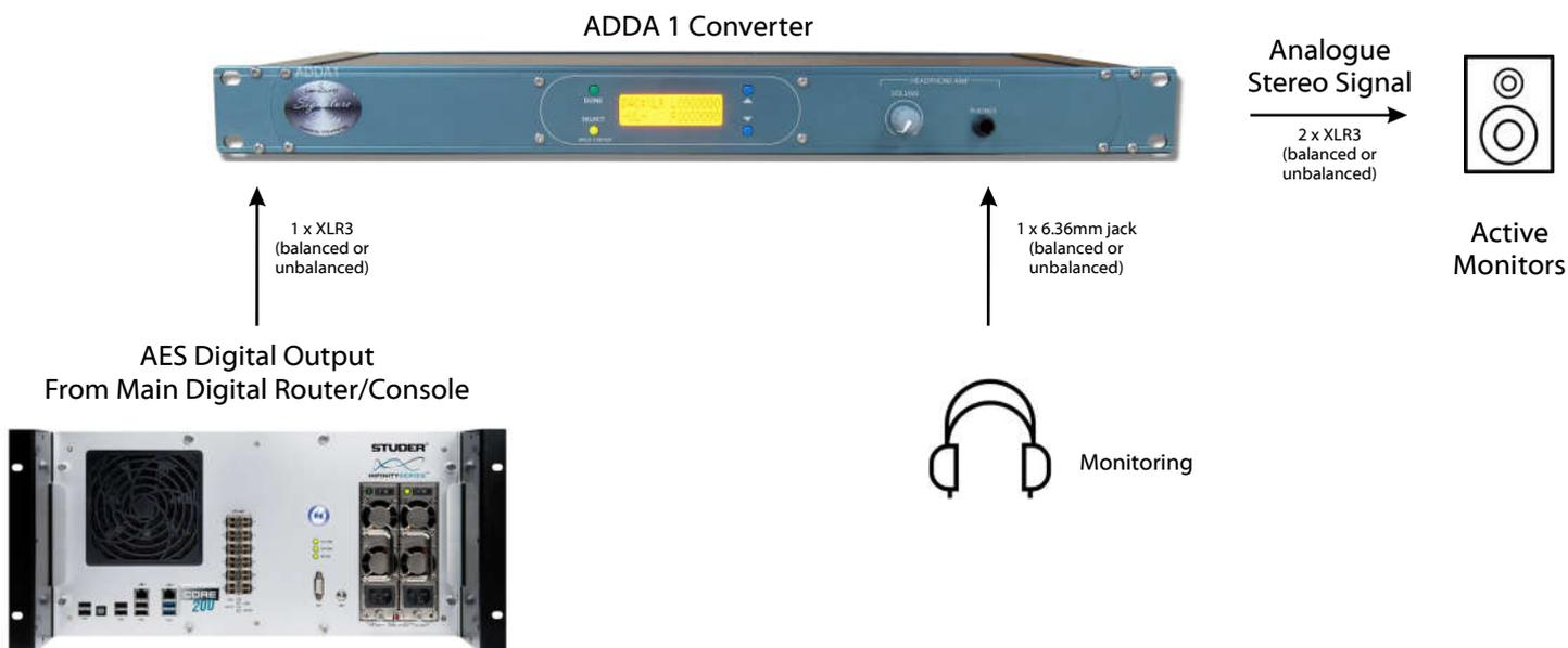
If a broadcast facility largely contains digital connections and you need to connect monitors to a studio, you will need a suitable analogue output.
