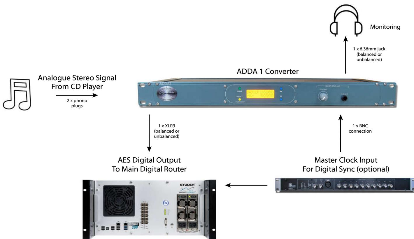
A radio station may be largely digitally linked, with all router and mixer connections via AES. If there are no analogue inputs on the system then the Signature ADDA1 can be used to link the CD player into the digital console.
