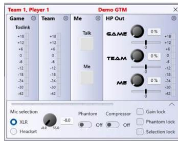
Adjust the incoming microphone gain via the XLR or headset connection. The GlenSound Referee compressor is automatic and prevents clipping, but a further compressor can be added to level out the audio signal. A meter will show real time input level.
