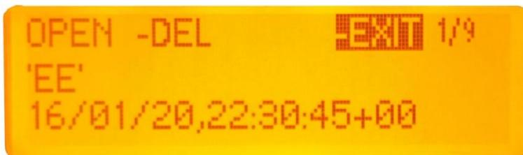
Along the top of the display are 3 options: '*OPEN*', '*DEL*' and '*EXIT*'. The x/X numbers after '*EXIT*' show how many texts you have received and the number of the text that you are currently viewing.
