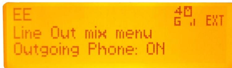
The first setting within the Line out mix menu is '*Outgoing Phone*' this option allows you to route what you are sending the outgoing phone (i.e. the output of the 2 audio input channels) to the Line Output. The options for this are 'ON' or 'OFF' to select between the 2 options use the navigation left and right arrows and once the desired option is selected press ENTER to set.
