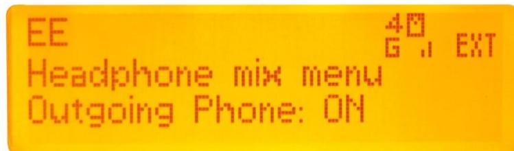
The first setting within the Headphone mix menu is '*Outgoing Phone*' this option allows you to route what you are sending the outgoing phone (i.e. the output of the 2 audio input channels) to your headphones for monitoring. The options for this are 'ON' or 'OFF' to select between the 2 options use the navigation left and right arrows and once the desired option is selected press ENTER to set.
