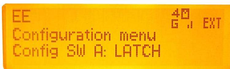
There are 4 options for A Switch Configuration which change how the front panel push switch that turns audio channel A on/ off to the output operate.
