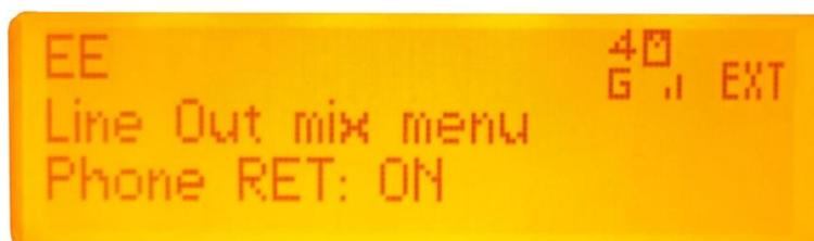
The last option in the Line out mix menu is '*Phone RET:*' This allows the option of routing the Return audio to the Phone ON or OFF to the Line out.
