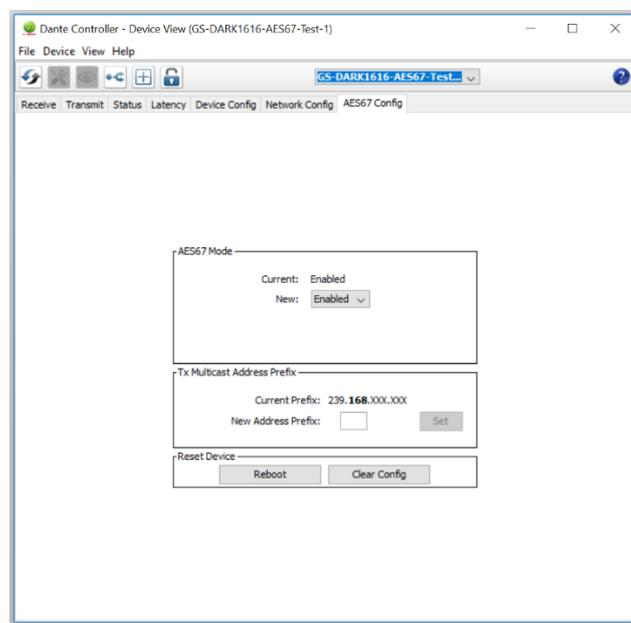
Once the AES67 drop down box has been enabled you'll have to reboot the Beatrice for the change to take effect. After the reboot go back to the AES67 tab and set the multicast prefix address to one that is suitable for your network.
