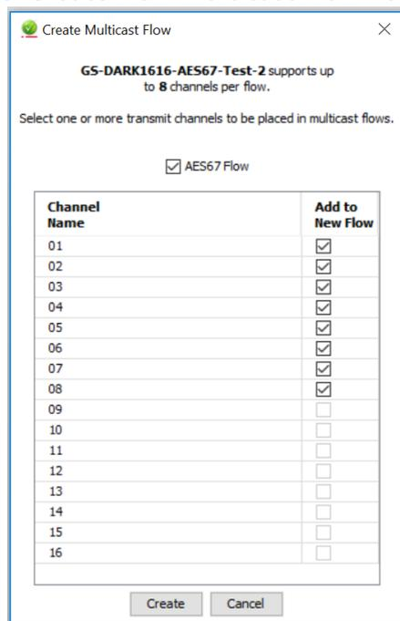
Tick the AES67 Flow check box, then select up to 8 channels to be included in the flow then click 'Create'
