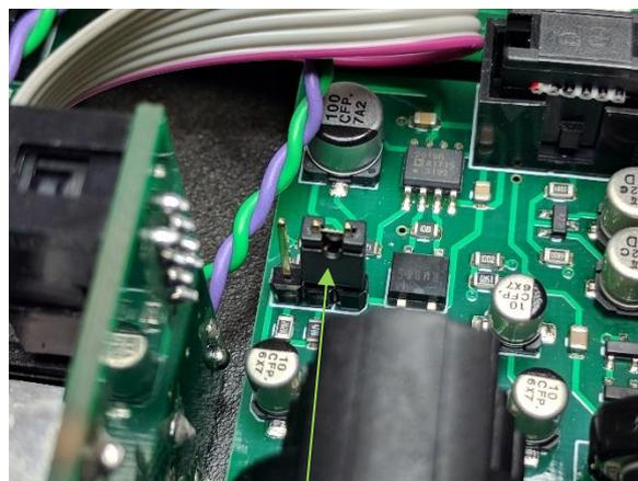
Jumper for Phantom Power ON
