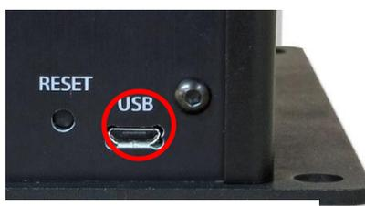
Figure 2 Left panel USB connector
