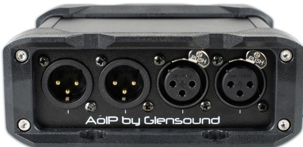
provides 2 analogue line level (0dB) inputs to the Dante® network and 2 analogue line level (0dB) outputs from the Dante® network. These circuits are electronically balanced on XLRs but can be wired unbalanced.
